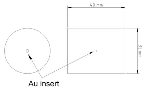
Schematic drawing of the phantom
