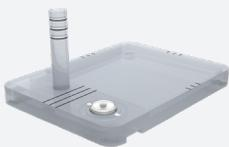
**Optional:** QUASAR™ Penta-Guide Tilt Plate is used to verify Image-Guided shifts for Six Degrees of Freedom Couches
