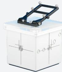
**Optional:** QUASAR™ Hood is used to confirm that the Varian Frameless Array or other visual position indicator is aligned with the CBCT and OBI
